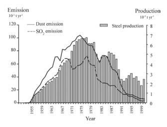
Fig. 2. Steel production, dust and  $SO_2$  emissions from the steelwork from 1954 to 2000.
